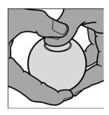
Battery Change Instructions: Remove switch plug and L.E.D. module. Then remove and replace batteries with 2x 2016 3v or DL2016 3v + side up. Reassemble.
